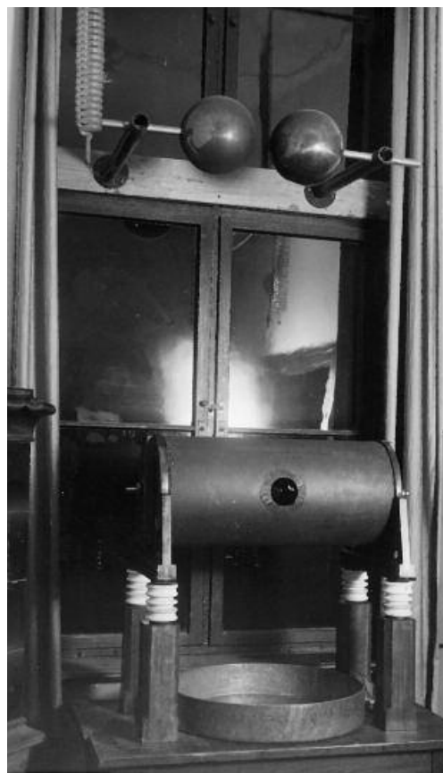
154. High-power vacuum tube with leaden protective casing
